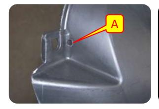
Once you have the rear trimmed to your liking, drill a 1/4" hole in the front of the inner fender. The hole should be in the corner of the front feature, roughly parallel to the stock hole [A].
