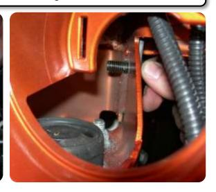
Step 5: Install MetalCloak Overline Fender Flares
