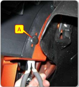
There is one plastic rivet [A] on the front of the Stock Fender Flare that needs to be removed. You can cut it off if you do not have a Plastic Rivet Removal Tool readily available.
