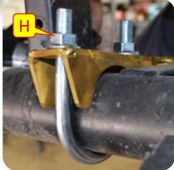
**Note:** It is helpful to have someone push the vehicle to the driver or passenger side to help align the hole; if you don't have an extra pair of hands you can use a ratchet strap on the frame/axle to pull the frame in the desired direction. Check to ensure the axle is centered once the bolt is in place. If not then remove the bolt, adjust the Track Bar length, replace the bolt, and re-check axle centeredness. Repeat until the axle is as close to center.
