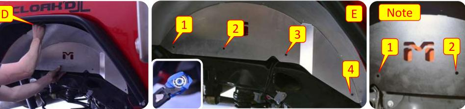
**Important Note:** *MetalCloak Recommends applying tape to a* 7/16 wrench to hold the nut in place during installation.
