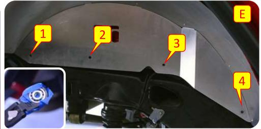
Important Note: MetalCloak Recommends applying tape to a 7/16 wrench to hold the nut in place during installation.
